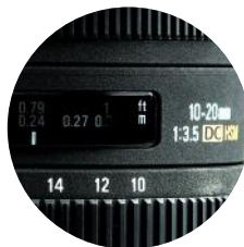
A Hyper Sonic Motor sets the focus quickly and quietly.
